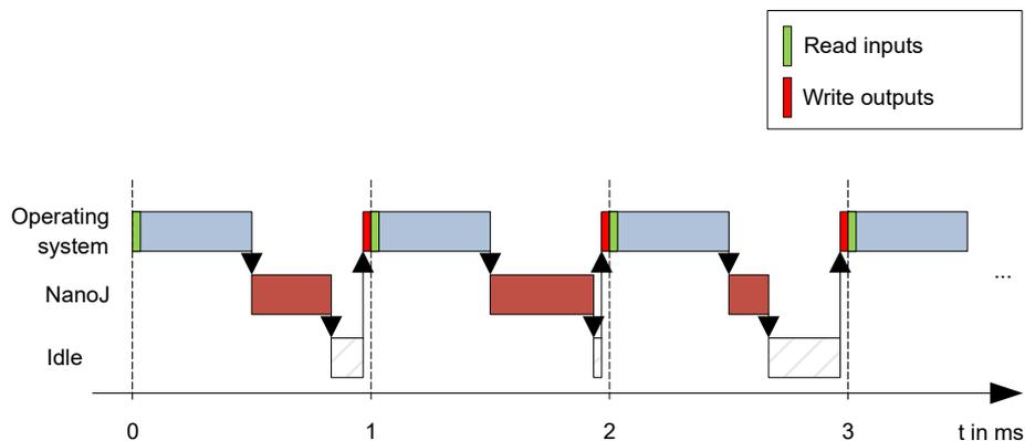
If the *NanoJ program* needs more time than was allotted, it is ended and an error code set in the object dictionary.
