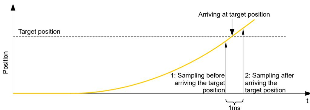
The current position is sampled once per millisecond. It is possible that the target position is reached between two samples. If the final speed is not equal to zero, then, after the target position is reached, the sample is used as an offset as the basis for the subsequent movement. As a result, the subsequent movement may go somewhat farther than expected.
