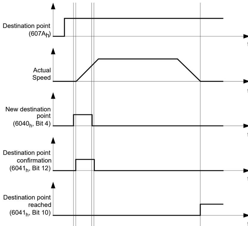
The controller can also reset bit 4 in object **6040<sub>h</sub>** (controlword) on its own. This is set with bits 4 and 5 of object **60F2<sub>h</sub>**.
