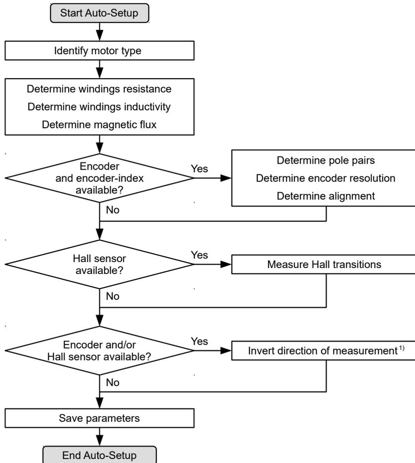
While the auto setup is running, the following tests and measurements are performed in succession:
