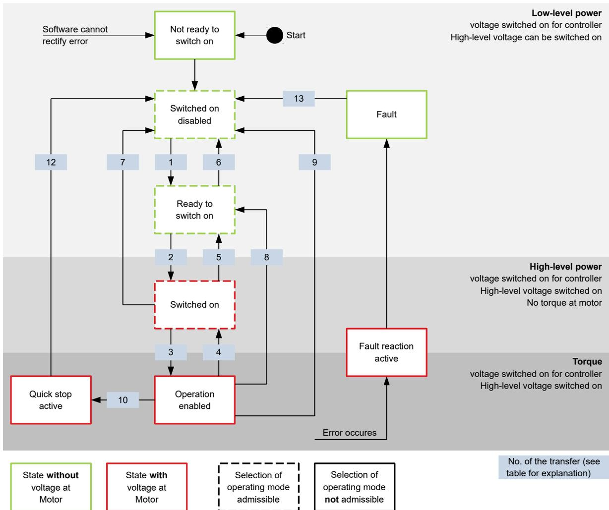
Listed in the following table are the bit combinations for the controlword that result in the corresponding state transitions. An X here corresponds to a bit state that requires no further consideration. The only exception is the resetting of the error (fault reset): the transition is only requested by the rising edge of the bit.
