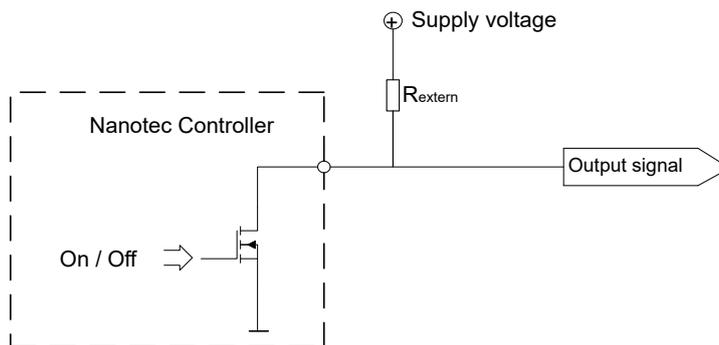
With a supply voltage of +24 V, a resistance value  $R_{\text{external}}$  of 10 k $\Omega$  is recommended.
