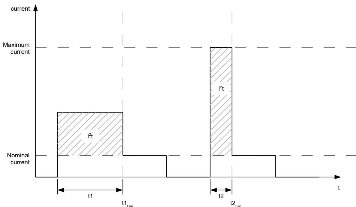
In the first section,  $t_1$ , the current value is higher than the rated current. At time  $t_{1Lim}$ ,  $I_{tLim}^2$  is reached and the current is limited to the rated current. A current that corresponds to the maximum current then occurs for a period of time  $t_2$ . Hence, the value for  $I_{tLim}^2$  is reached more quickly than in time  $t_1$ .
